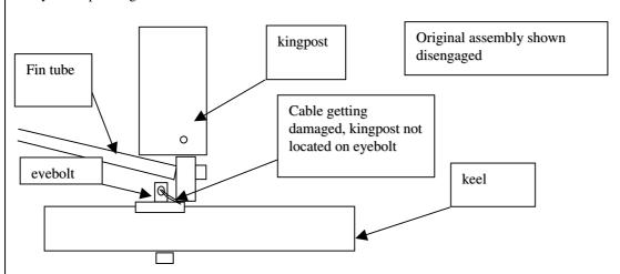
Although it is most probable that the kingpost disengagement happened during rigging, it is not inconceivable that taxiing over very rough surfaces or unusual flight manoeuvres might cause disengagement.
